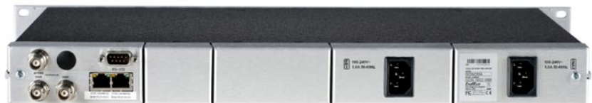
Sonoma rear panel with optional dual power supplies. Antenna input TNC connector on upper left. Two spare BNC connectors on lower left. One RS-232 connector. Two 10/100/1000Base-T Ethernet ports. Optional dual optional power supply connectors on right.
